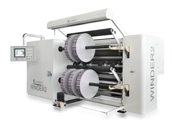
High performance machines for slitting and rewinding flexible materials
